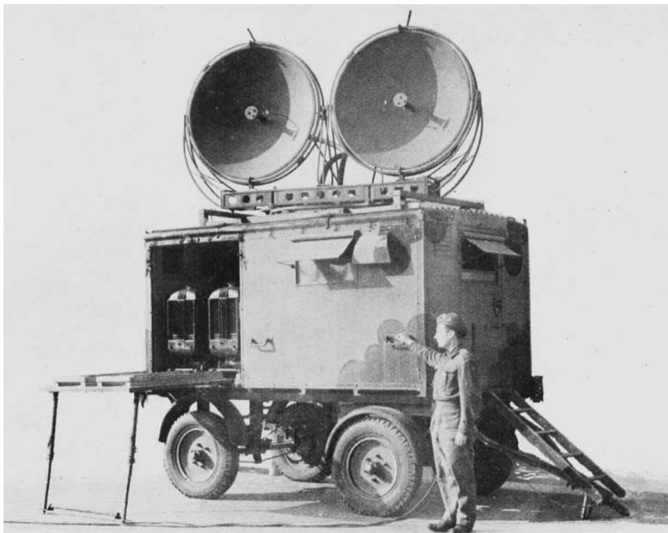
Fig. 9. Wireless Set No. 10 in Trailer
