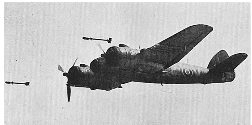
Fig. 12. A Beaufighter Firing a Pair of 60 lb. (High-explosive Head) Rockets
