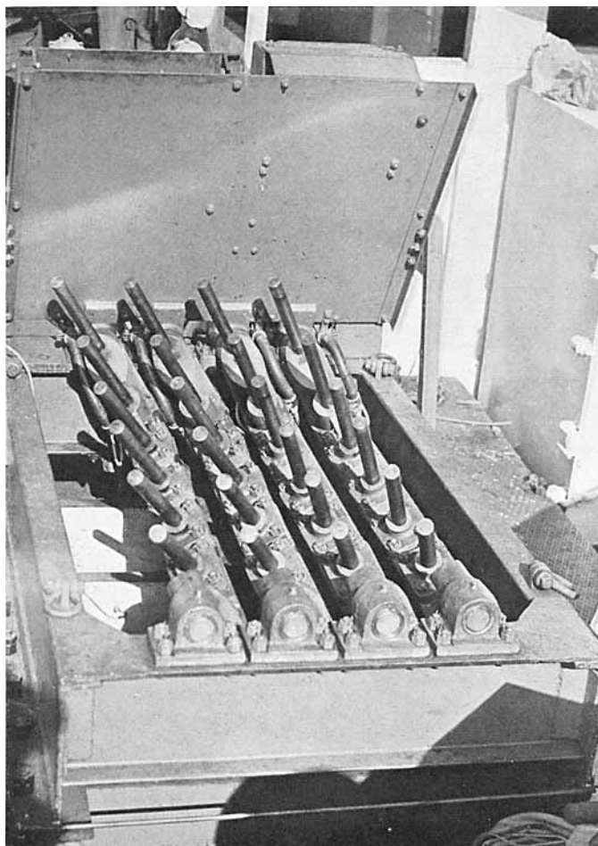
Fig. 53. Hedgehog Mounting trained to Starboard View taken before end covers were fitted to bearings.
