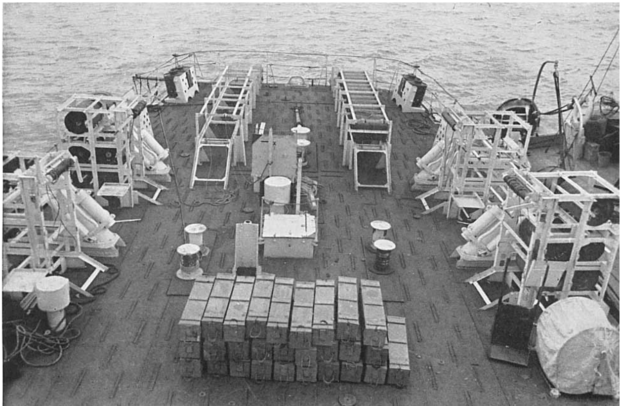
Fig. 39. Quarter-deck of Depth Charge Fitted Escort Vessel showing Launching Rails, Throwers, and Loading Racks for Depth Charges
