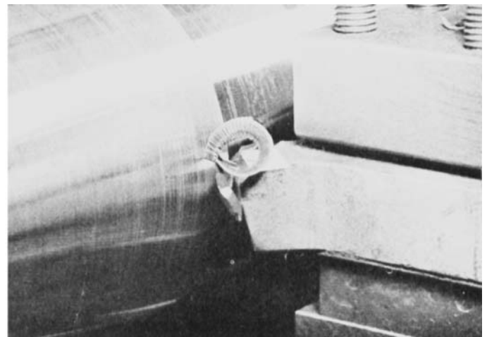
Fig. 14. Tool with 40 deg. Negative Rake
